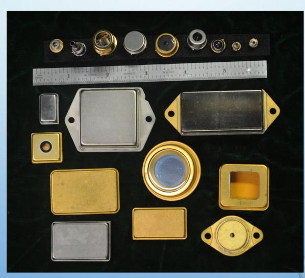
Below the ruler are larger packages that benefit from welding using low impedance welding technology
